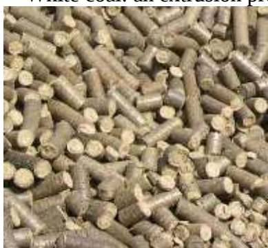
White coal: an extrusion product of groundnut shell ↓
