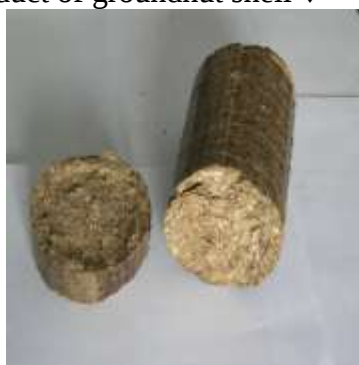
White coal: an extrusion product of groundnut shell ↓
